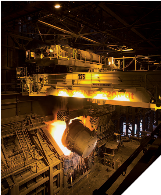
Crane performing charging task.
